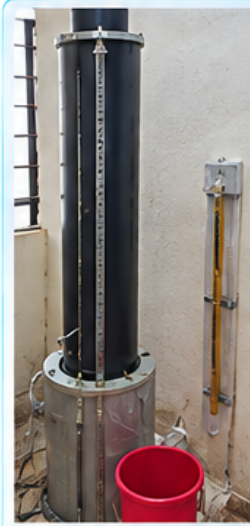
Variable Head Apparatus
