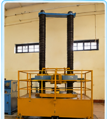
Column Testing Machine
