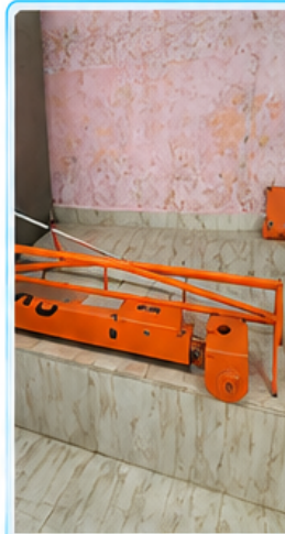
Benkelman Beam Deflection
